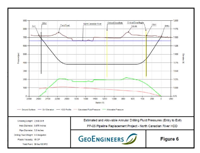
Attachment 3. Horizontal directional drilling profile.
